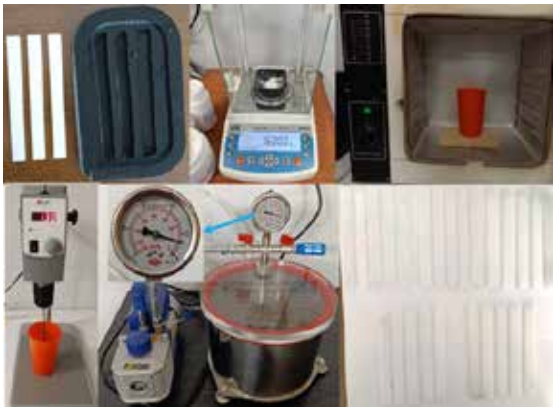
Figure 1. Schematic representation of the specimen fabrication steps followed in this study.
