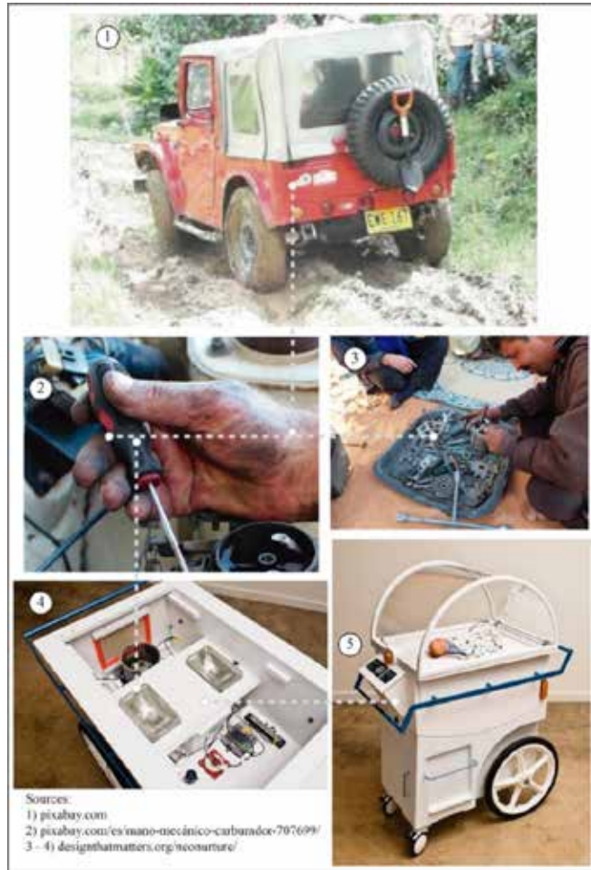
Figure 10. NeoNurture, incubator made with vehicle parts
